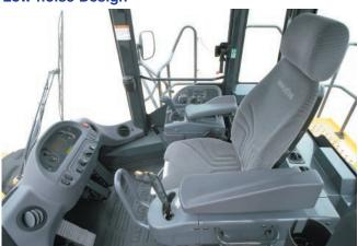
Noise at operator's ear noise level : 76 dB(A) Dynamic noise level (outside): 113 dB(A)
