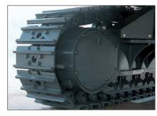
**Sturdy guards** shield the travel motors and piping against damage from rocks.
